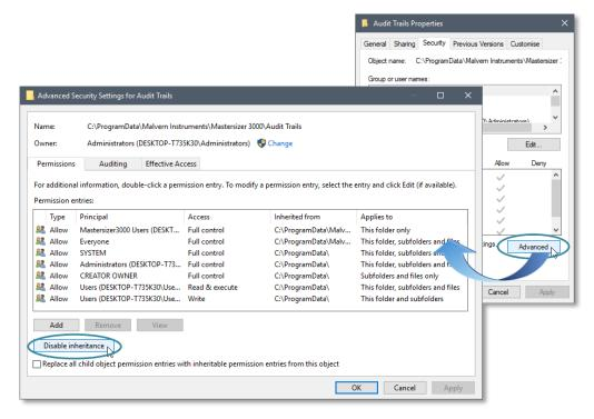
4. Within Block Inheritance, left-click on Convert inherited permissions into explicit permissions on this object – this removes the permission inheritance from the parent folder, whilst keeping the any current users and groups settings.
