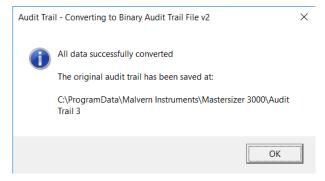
If you are upgrading from Mastersizer 3000 software v3.70 to v3.71 the message below will be displayed, indicating that an audit trail format update is being applied to fix bug issue #91576:
