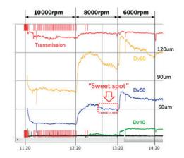
Real-time measurement system makes it possible to instantly observe the effect of decreasing the speed of rotation of the atomizing disk and the time taken for the process to re-establish a steady state. (Green Dv10, blue Dv50, orange Dv90, red is transmission).
